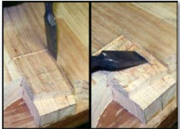
Figure 9 Defining the area with stop cuts helps prevent overshoot when you cut across the grain
