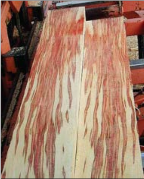
Boards of box elder, sometimes called “flameboards”
