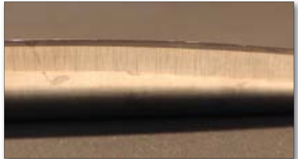
Figure 3 The glint along the edge, seen from the side of or directly above the edge, signals the need for sharpening.
